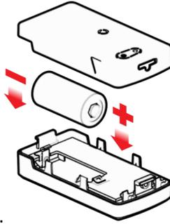
3. Insert the new battery as shown.
