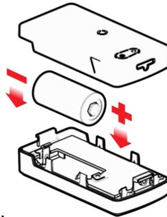
3. Insert the new battery as shown.
