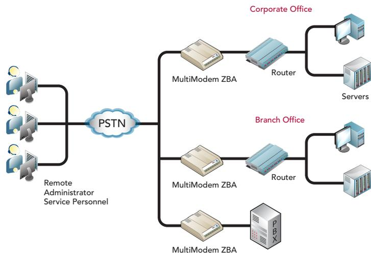
The above diagram represents a typical Out of Band environment using Multi-Tech MultiModem ZBA (MT9234ZBA-IEC-OBM) modems to remotely manage routers and PBXs.
