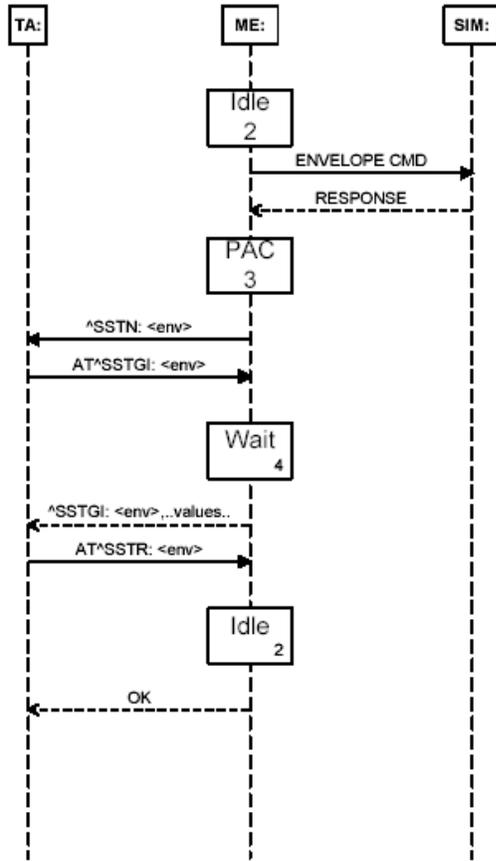
Envelope commands are issued for Call/MO control by the SAT if Call control is enabled. Upon receiving the response from the SIM application, SAT changes to the PAC state.
