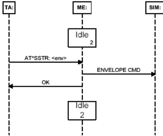
A SIM application will provide SAT with a main menu to display, using the PAC SETUP MENU. The envelope command MENU SELECTION allows the TA to select an item from this menu using AT^SSTR.
