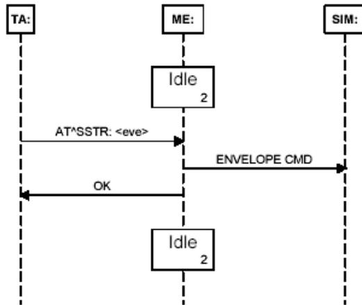
When an event occurs that is in the TA event list, as configured using the PAC SETUP EVENTLIST, SAT is informed using AT^SSTR.
